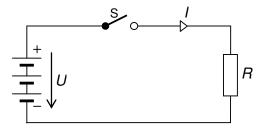
An **electrical network** is an interconnection of electrical components such as resistors (R), inductors, capacitors, or their combinations, voltage sources (U), current sources, and switches (S) with transmission lines.
